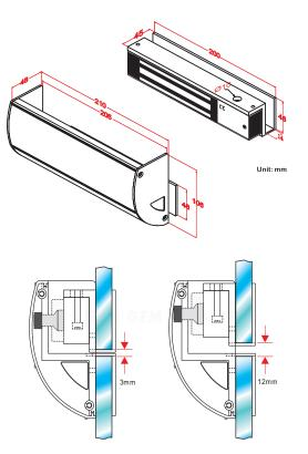
The thickness of glass should be 10~13mm and the armature plate can be adjusted depending on the door gap ranging from 3mm to 12mm.
